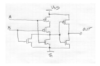
c) Design the CMOS circuit (referred to as a "compound, static gate") that realizes the function:
